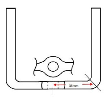
Bend the required bends. Centre of the bend desired should be 35mm from the centre of the punched hole. Prepare ends of bar for fire welding.
