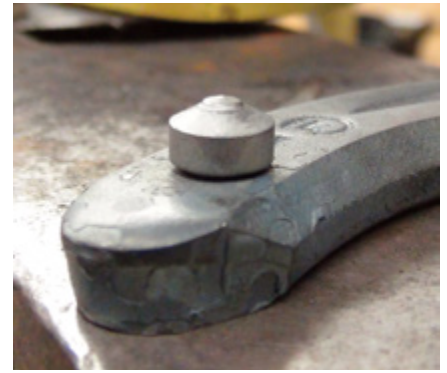
C11 applied – note the small gap between head and shoe surface.
