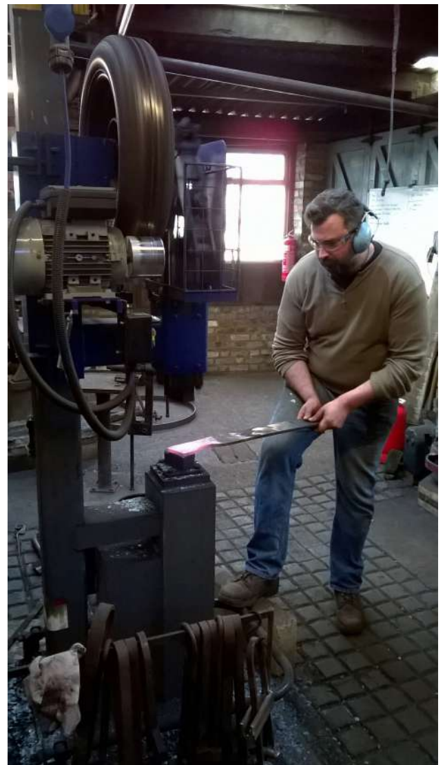
Doug Campbell at work forging part of the detailing for a panel ►
