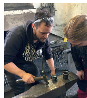
A blacksmith makes a crotal bell, also known as rumble bells, which were used on horse-drawn vehicles before motorised vehicles were common
