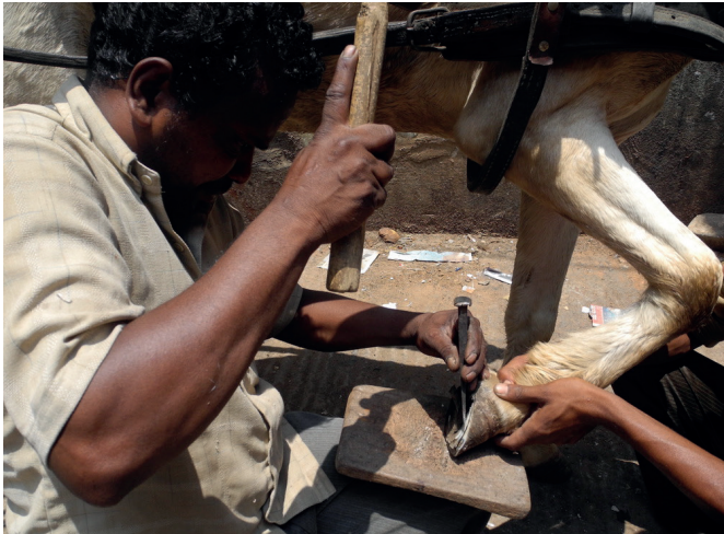
Azam at work, using a wooden board on his knee and a chisel for trimming
