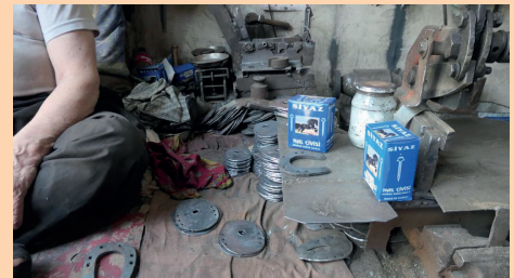
Blacksmiths in Tabriz produce plate shoes for horses that work on stones and rocks in the mountains
