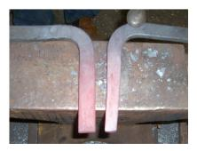
The steel is also narrowed in preparation for the setting down and graduating of the branch.
