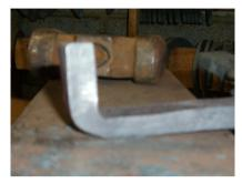
Forge the top of the caulkin down. This starts the shaping of the caulkin. Only allow yourself 3 blows on each different angle of the caulkin. The reason I count the three blows is to reduce the chance of over working one particular side of the caulkin. There are five positions to forge the caulkin -
