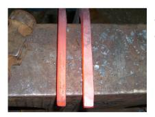
The drawing down creates a squarer section. Notice the thickness created compared to that of the undrawn branch.
