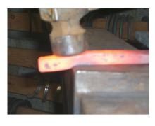
Now set approximately 1.75 inches over a round edge. Then run back up the branch towards the toe with overlapping blows. One run is enough at this stage.
