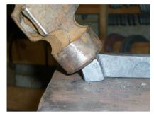
The fifth position comes after a heat so that the caulkin will turn easily to bring the face of the caulkin in line with the toe. Hold the branch at 45 degrees to the anvil, make sure hammer blows are parallel to the edge of the anvil and work the caulkin back. You can also set the caulkin down over the sharp edge of the anvil at the same time and work back up the branch towards the toe to get the necessary graduation, shown here -
