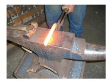
Always ensure you have the correct heat, the steel in this case 1 inch x 0.5 inch needs to be white or to put it another way 'dripping'.
